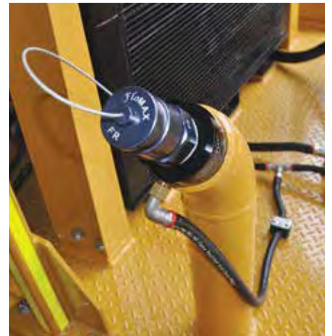
Fast fuel filling connection and fuel level indicator
