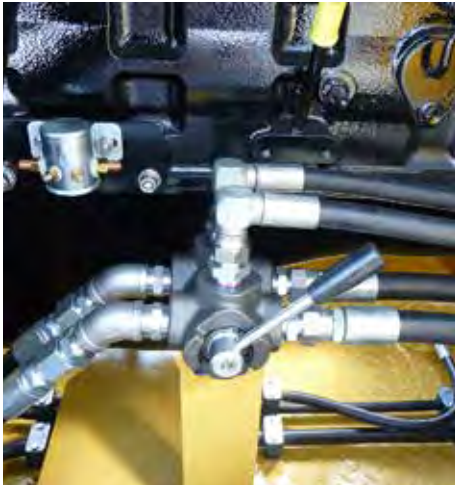
3 Way fuel control systems for multiple supply tanks
