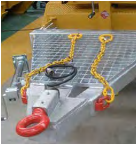
Heavy duty drawbar and safety chains
